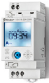
Type 12.A1.8.230.0000 1 wisselcontact, 16 A 110...230 V AC/DC
