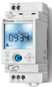
Type 12.61.8.230.0000 1 wisselcontact, 16 A 110...230 V AC/DC
