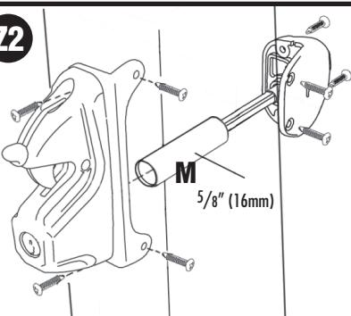
Insert PVC tube M for vinyl and wood fence posts.
