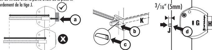
**8 Attach bush F onto back of latch B.**
