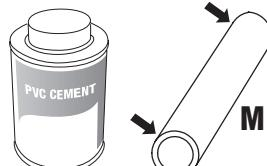
Apply glue completely around edges of PVC tube on both sides of fence post
