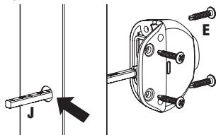
**7 a) Push rod J in towards the post to fully extend the button outwards.**
