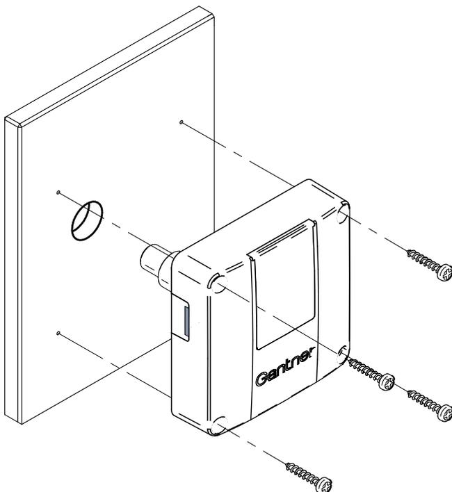
**(Eng)** For wooden or HPL doors: 05x35 mm (03/16"x1-3/8") pan head wood screws (stainless steel A2).
