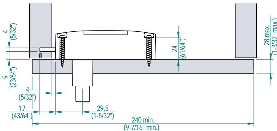
Ⓜ The distance of 4 mm (5/32") indicated between the lock housing and the locker body is valid for locker doors that are wider than 240 mm (9-7/16") and with a maximum door leaf thickness of 28 mm (1-3/32"). For locker doors that do not adhere to these measurements, or for doors with an unfixed pivot point (depending on the type of hinge used), the distance between the lock and the body of the locker must be recalculated.
