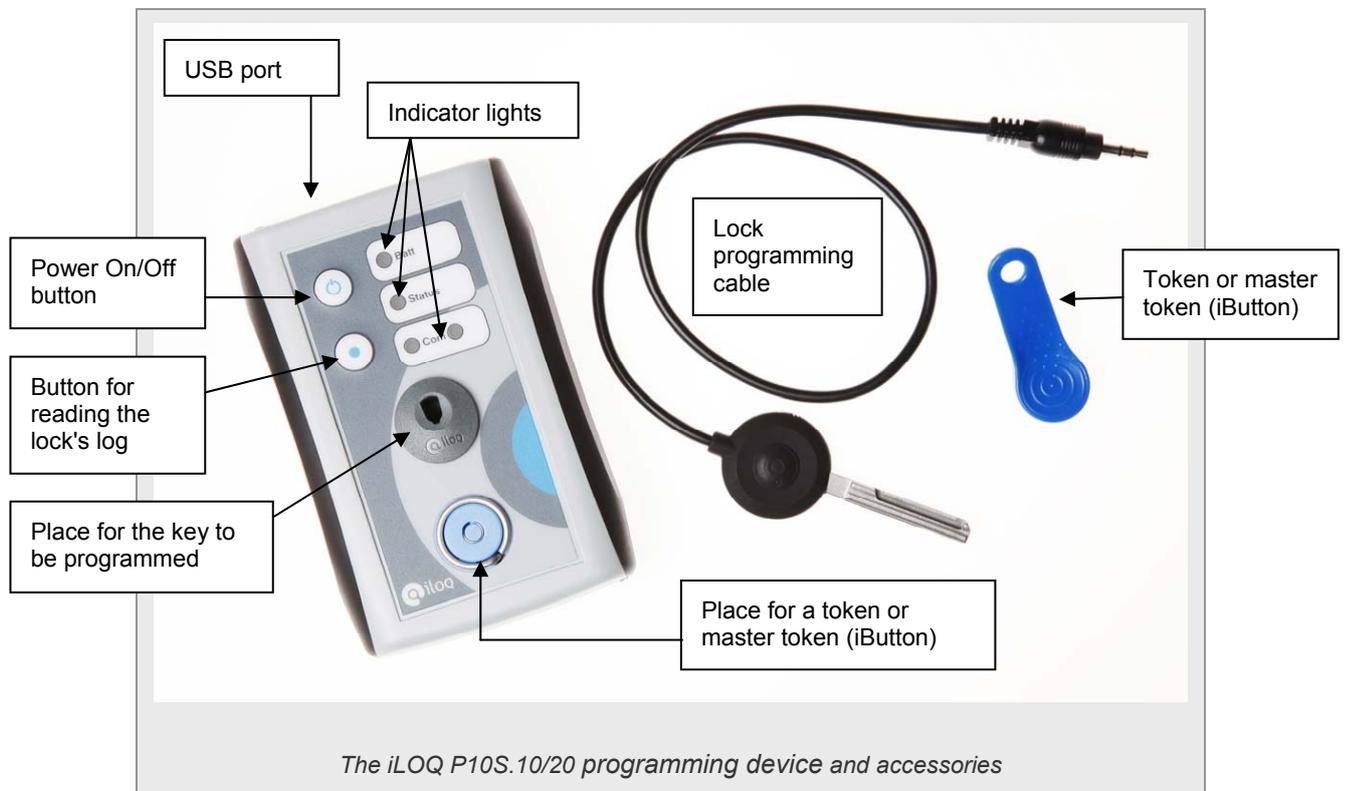
The front panel of the programming device contains a keyhole for the key to be programmed and a receptor for an iButton®, also called a token or master token. The iButton contains data of the locking system's security mechanisms, and it must be connected to the programming device while programming both locks and keys.
