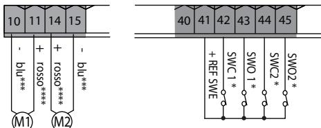
**VIRGO SMART BT A (3 fili - 3 wires - 3 fils - 3 Drähte - 3 cables - 3 fios)**t iPo RotorE - tYPE dE RotorEur - RotorEntYP - Rotor tYPE - t iPo Rotor: **10**
