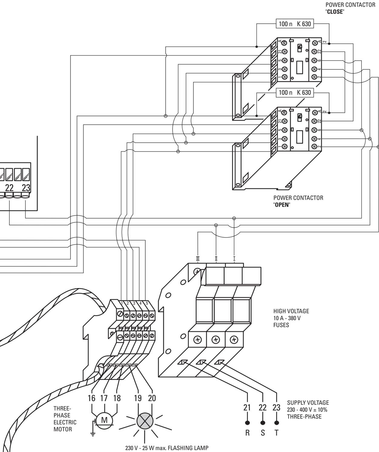
The electronic control panel Elpro 10 Plus, new generation, is designed to operate the sliding gates. Power supply is 230/400V three-phase. Built in full compliance with BT 93/68/CE Low/High Voltage and EMC 93/68/CE Electro-Magnetic Compatibility Regulations. Fitting operations are recommended by a qualified technician in conformity to the existing safety standards.
