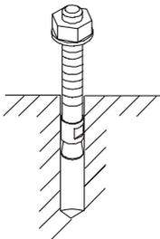
BORE 4 HOLES IN KEEPING WITH THE DIAMETER OF THE PLUGS AND THE PASSAGE
