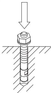
INSERT THE PLUGS IN THE HOLES LEAVING A PART PROTRUDING FROM THE FLOOR EQUIVALENT TO THE THICKNESS OF THE BASE PLATE AND FIXTURE NUT, CONSIDERING THE PROTRUSION OF THE PLUG DURING TIGHTENING
