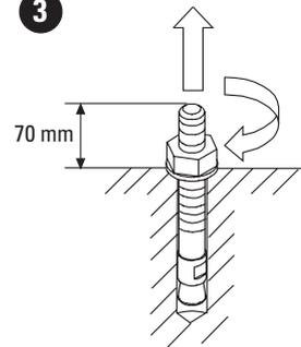
TIGHTENING THE PLUGS: ONCE THE PLUG PROTRUSION HAS BEEN ESTABLISHED, TIGHTEN THE NUT TO THE FLOOR IN ORDER TO FIRMLY FIX THE PLUG IN THE HOLE, THEN UNSCREW AND REMOVE THE NUT
