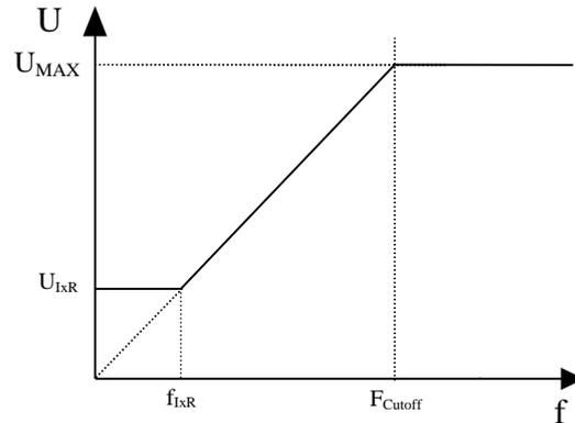
Figure 3 IxR compensation characteristic curve
