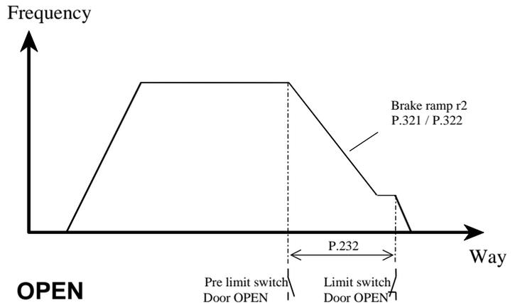
**Figure 9 Pre-limit switch position Door OPEN**
