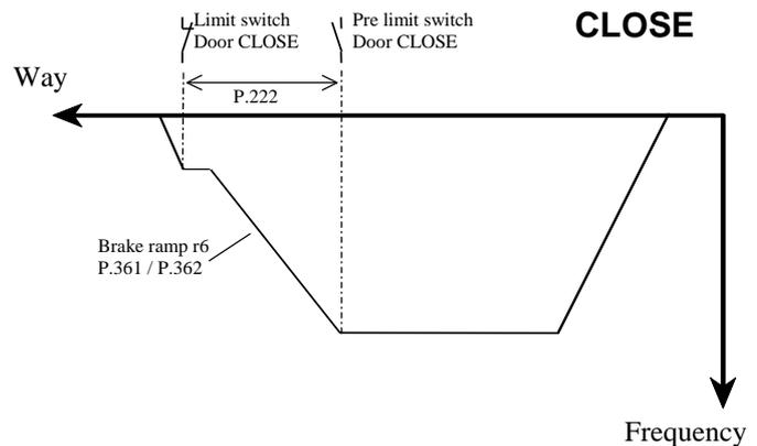
Figure 6 Pre-limit switch position Door CLOSE
