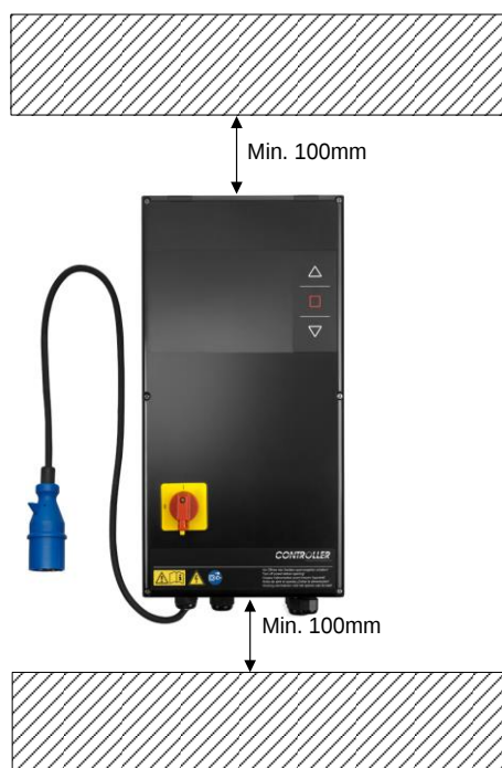
Figure 1: Installation de la commande
