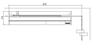
Space required on doors for standard installation on hinge side
