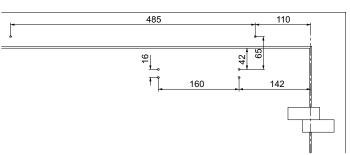
Installation dimensions for direct standard mounting on hinge side Right handed door shown in diagram Left handed door is the reverse
