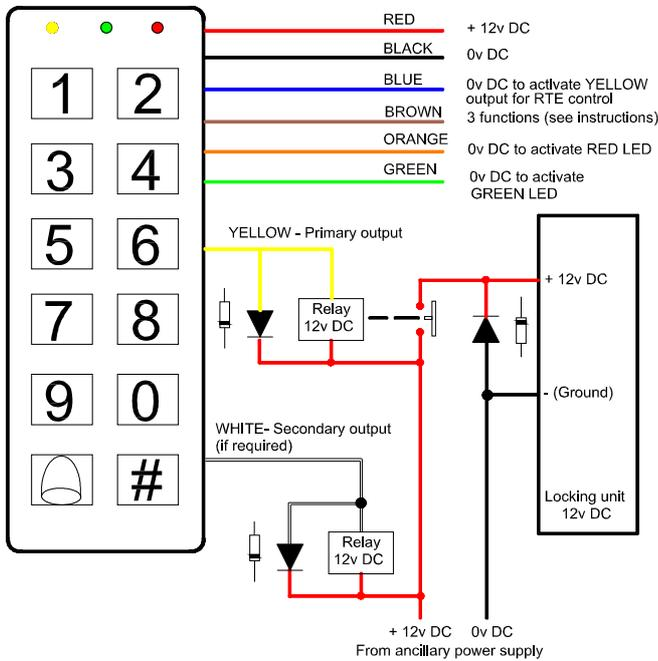
Locking unit, supplementary relays and additional diodes shown in the above circuit diagram are for illustrative purposes only and are not included with the CT1000. Please order separately.
